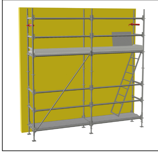
Projeye göre iskele sistemi cepheye ankrajlanır. The system is anchored to the facade according to the scaffolding drawings.
